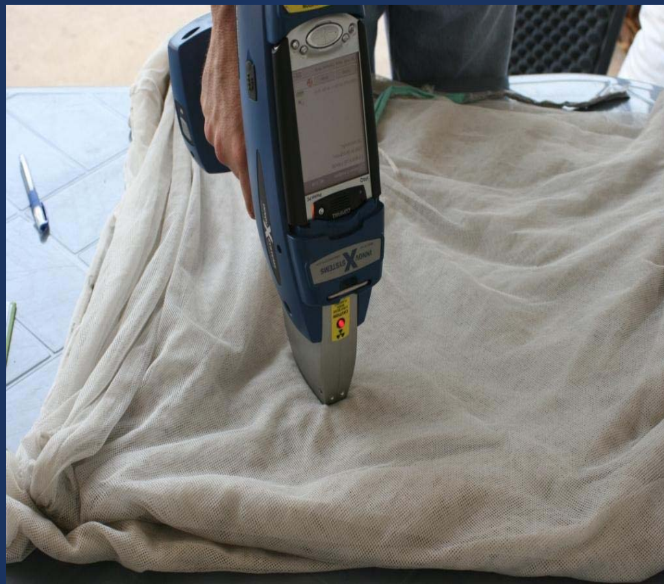
X-ray fluorometer - deltamethrin in PermaNets (Photo: S. Smith)
