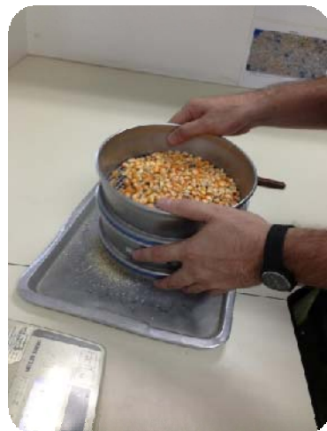
Grading corn-Seiving-defected, damaged, cracked, rotten, fine
