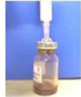
Inject the diluent with sample in to Magnetic nano particle container
