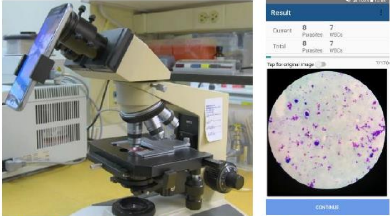
Fig. 7. Smartphone-based malaria data acquisition and parasite detection.
