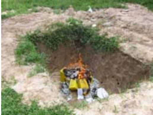
Fig 1—Burning test of safety box filled with used AD syringes.
