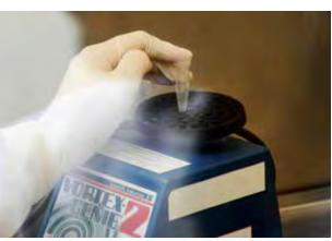
↑ A vortex mixer is used in the lab to mix small vials of liquid
