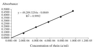
Fig 2–Calibration curve of rhein in 0.5% magnesium acetate solution in methanol determined by UV-vis spectrophotometric method.
