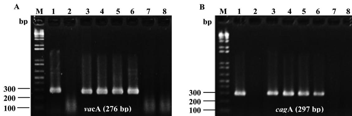
Fig 4—Agarose gel-electrophoresis of *H. pylori vacA* (A) and *cagA* (B) amplicons using nested-PCR. Amplification conditions are described in Materials and Methods and Table 1. Lane M, 1 kbp DNA size markers; lane 1, positive control; lane 2, negative control; lanes 3-8, saliva samples of asymptomatic subjects.
